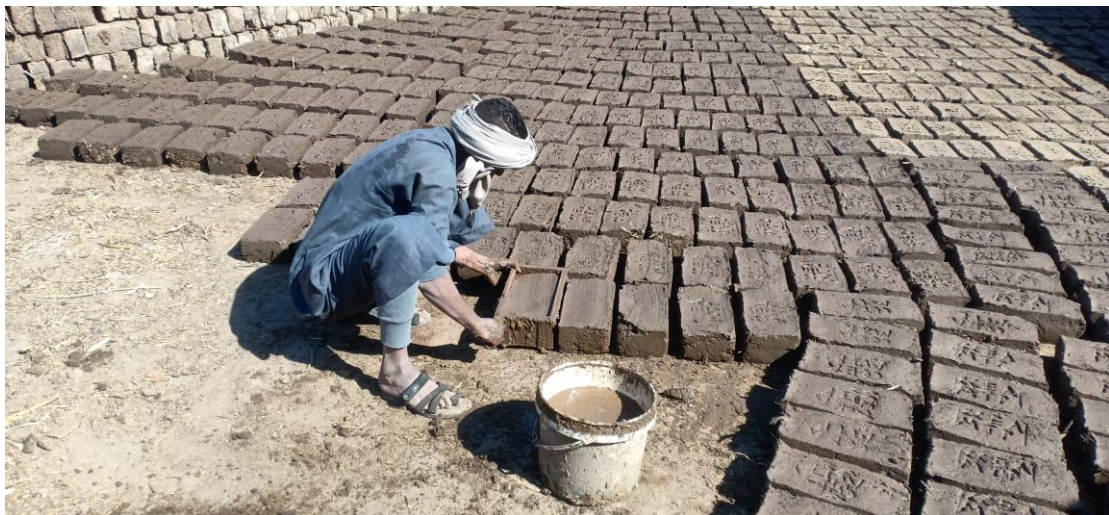
Fig. 16 Processes of making Mud-bricks © MTP
