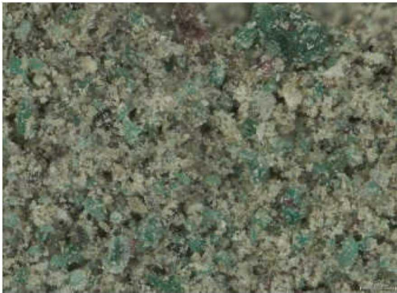
图五八 样品 M17:1-2, Cu: 11.4%, Sn: 35.98%, Pb: 43.93%, 含大量白铅矿
