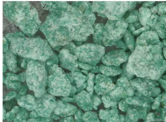
图五六 样品 M18:7-2, Cu: 86.34%, Sn: 12.88%, Pb: 0.33%
